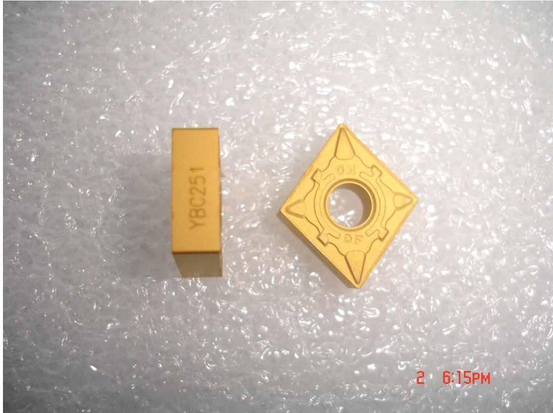
CNMG-DF YBC 251 P10-P30 SEMI-FINISHING FOR STEEL
